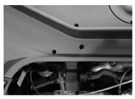
7. Install the cover and place the Lifting System conduit as shown in the figure.
