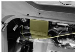
8. Fix the cover to the cowl cover with the screw provided in the kit.
